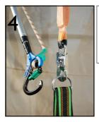
Extend pole, reach down and attach the karabiner to the main anchor point on the casualties harness. Once located you can pull away the pole.
