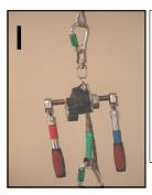
Hang device on an anchor point or suitable load bearing coupler above or as close to the casualty as possible.
