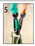
Ensure connection is to the anchor point On the harness and not the webbing.
